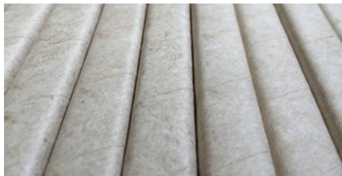
Rectangular conductor insulated with aramid-enhanced cellulose paper DuPont™ Nomex® 910 (photo by DuPont)
