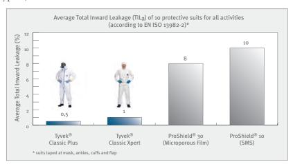
EN 1073-2\*\* measures the inward leakage of particles into the whole suit. The result is then expressed as the Nominal Protection Factor (NPF) of a garment. Tyvek\* Classic Plus and Tyvek\* Classic Xpert meet the requirements of Class 2 (NPF > 50), whereas most other Type 5 protective suits are only Class 1 (see table below).
