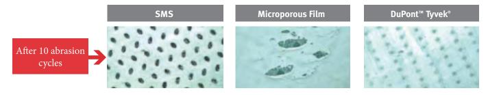
Beyond its high abrasion and tear resistance, Tyvek° is also lightweight and soft, as well as permeable to both air and water vapour, providing a high level of wear comfort. Thanks to its smooth surface and antistatic treatment, Tyvek° prevents particles from adhering to the coverall.
