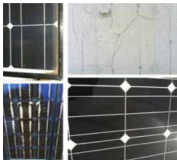
Figure 3. Representative visual defects (clockwise from top left): etched glass, cracked backsheet, snail trails and encapsulant discoloration.
