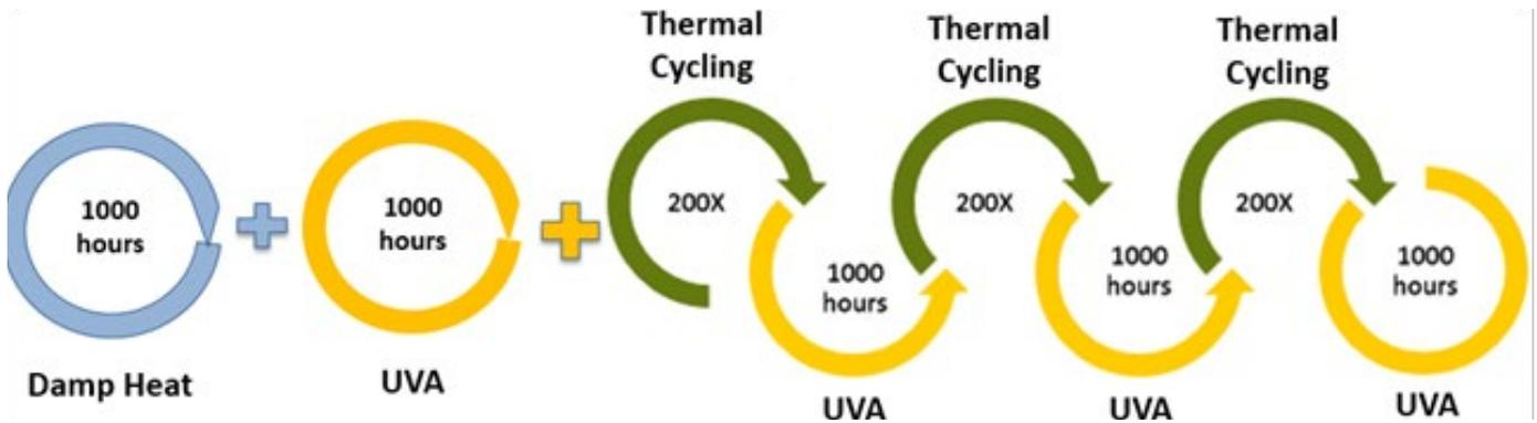
For example, the given sequential ageing test was conducted on PVF and PVDF based backsheets. After the test, PVDF backsheet cracked along transverse direction. This happened due poor mechanical properties of the PVDF film which becomes brittle after exposure to damp heat conditions (refer figure – shows complete loss of elongation
