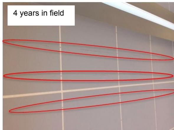
This is not a standalone case of backsheet cracking in China. By 2016 the industry began to hear about more and more cases of backsheet cracking in only 4-5 year old installations. Not only China, backsheet cracking instances have been found in less than 5-year old solar plants in Europe and Southeast Asia. Module manufacturer had to replace these modules under 10-year product warranty which caused huge financial losses
